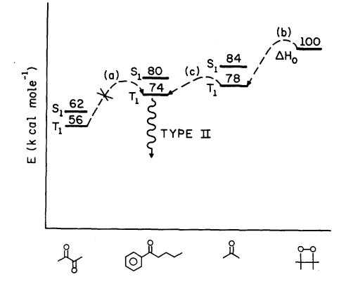
Figure 1. Energy diagram sketching the proposed mechanism of reaction 3. Direct excitation of  $T_1$  of valerophenone by biacetyl triplets (path a) is energetically unfavorable and not observed.  $T_1$  of biacetyl, however, is able to generate acetone triplets from the dioxetane (path b). Acetone triplets, in turn, sensitize formation of valerophenone triplets, which then undergo Type II reaction (path c).
